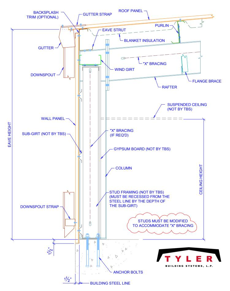
SIDEWALL SECTION OPEN FOR WALL MATERIAL BY OTHERS WITH WALL PANELS
