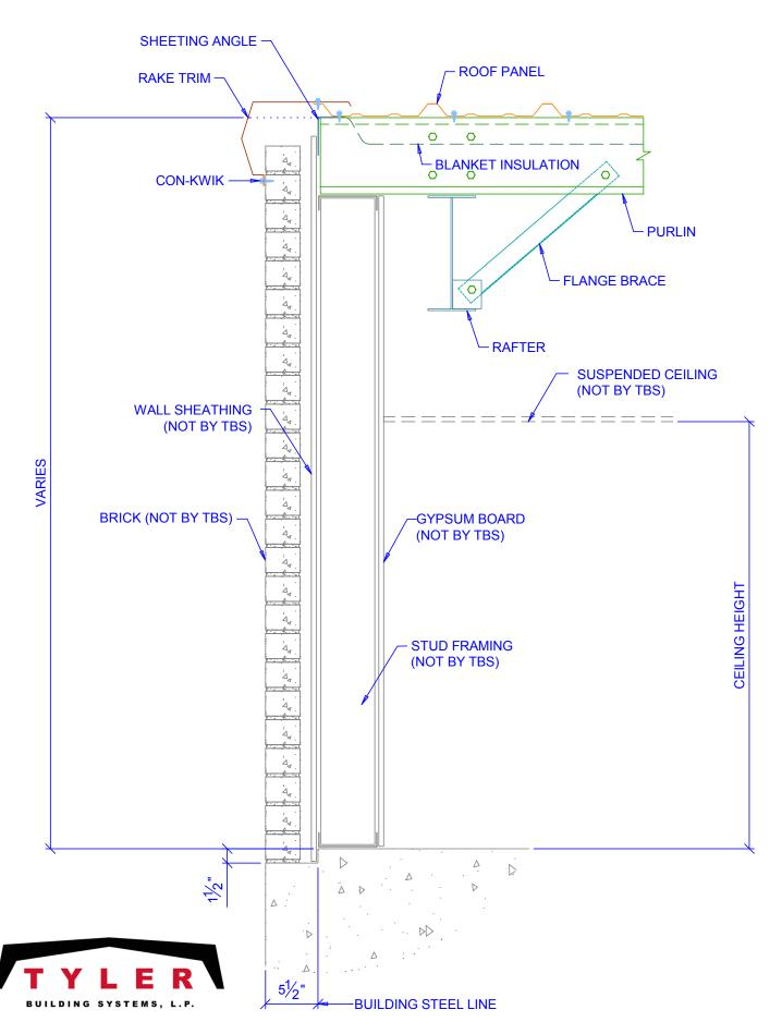
RIGID FRAME ENDWALL SECTION OPEN FOR WALL MATERIAL BY OTHERS
