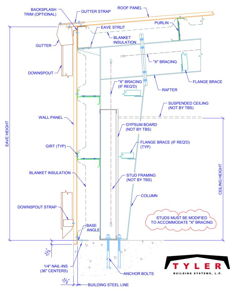
STANDARD SIDEWALL SECTION WITH STUD WALLS
