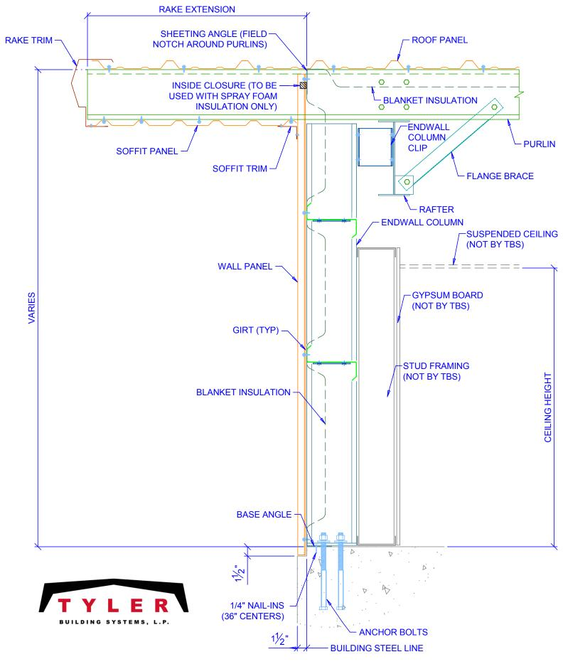
RIGID FRAME ENDWALL SECTION WITH STUD WALLS
