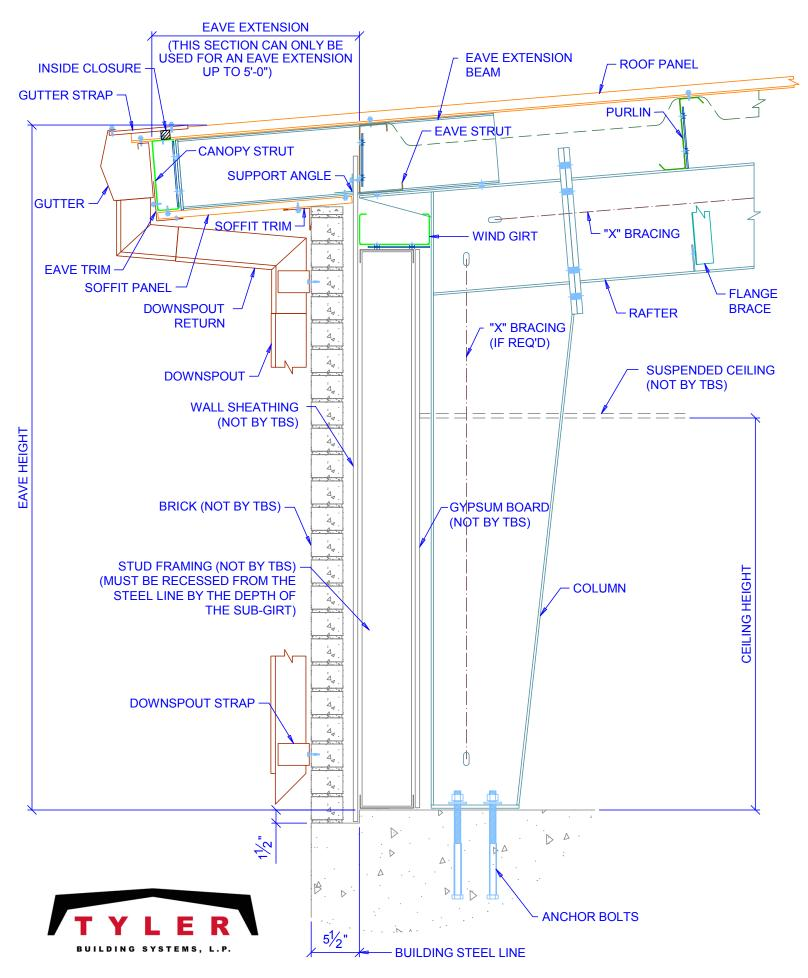
SIDEWALL SECTION OPEN FOR WALL MATERIAL BY OTHERS
