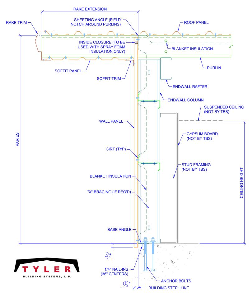
BEARING ENDWALL SECTION WITH STUD WALLS
