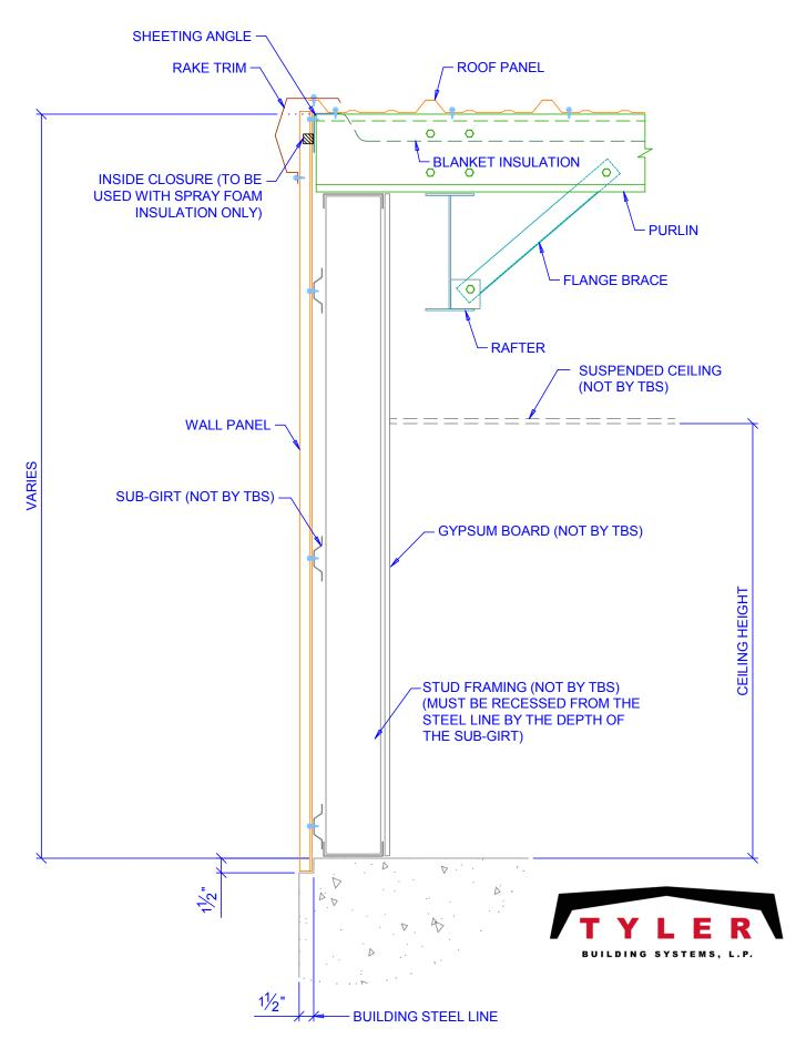
**RIGID FRAME ENDWALL SECTION OPEN FOR WALL MATERIAL BY OTHERS**
