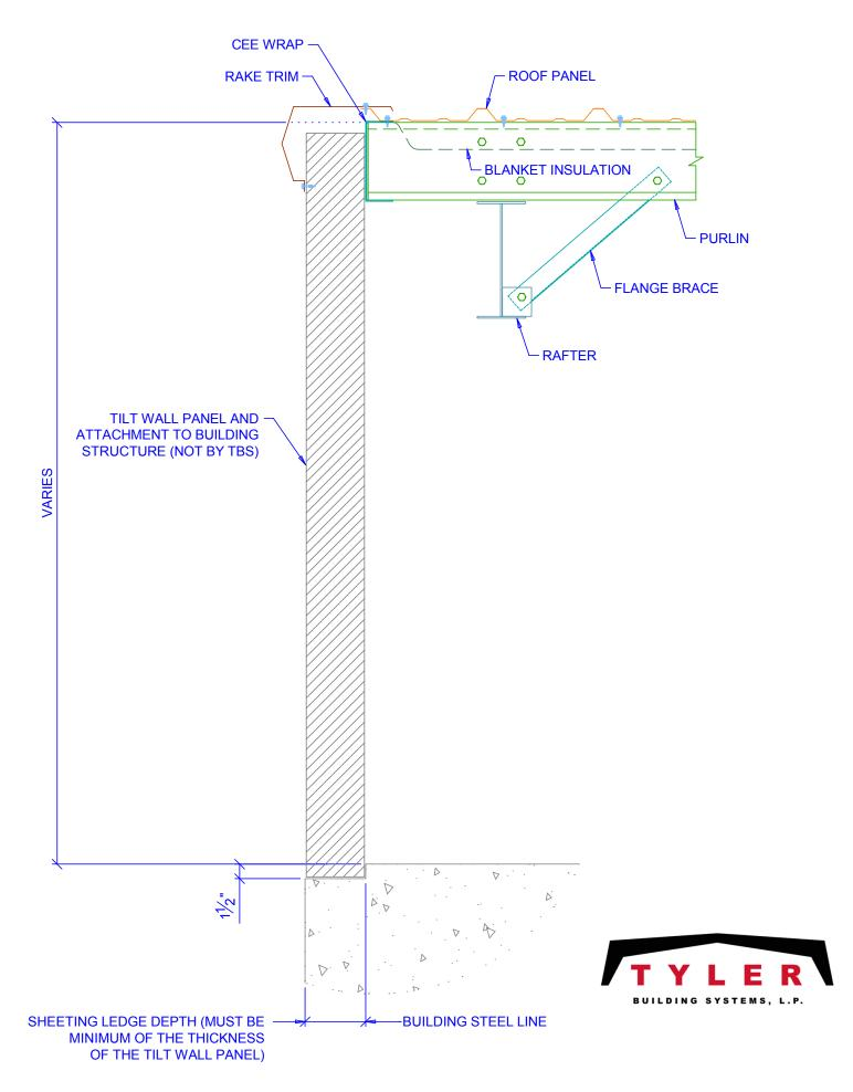
RIGID FRAME ENDWALL SECTION OPEN FOR TILT WALL
