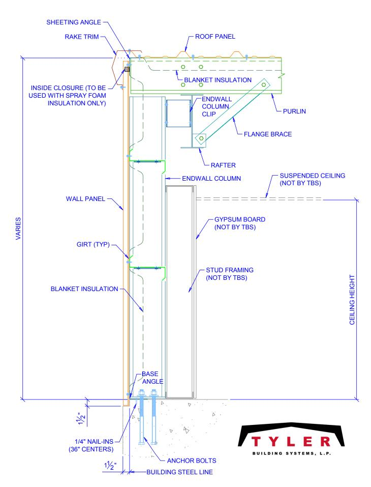
RIGID FRAME ENDWALL SECTION WITH STUD WALLS
