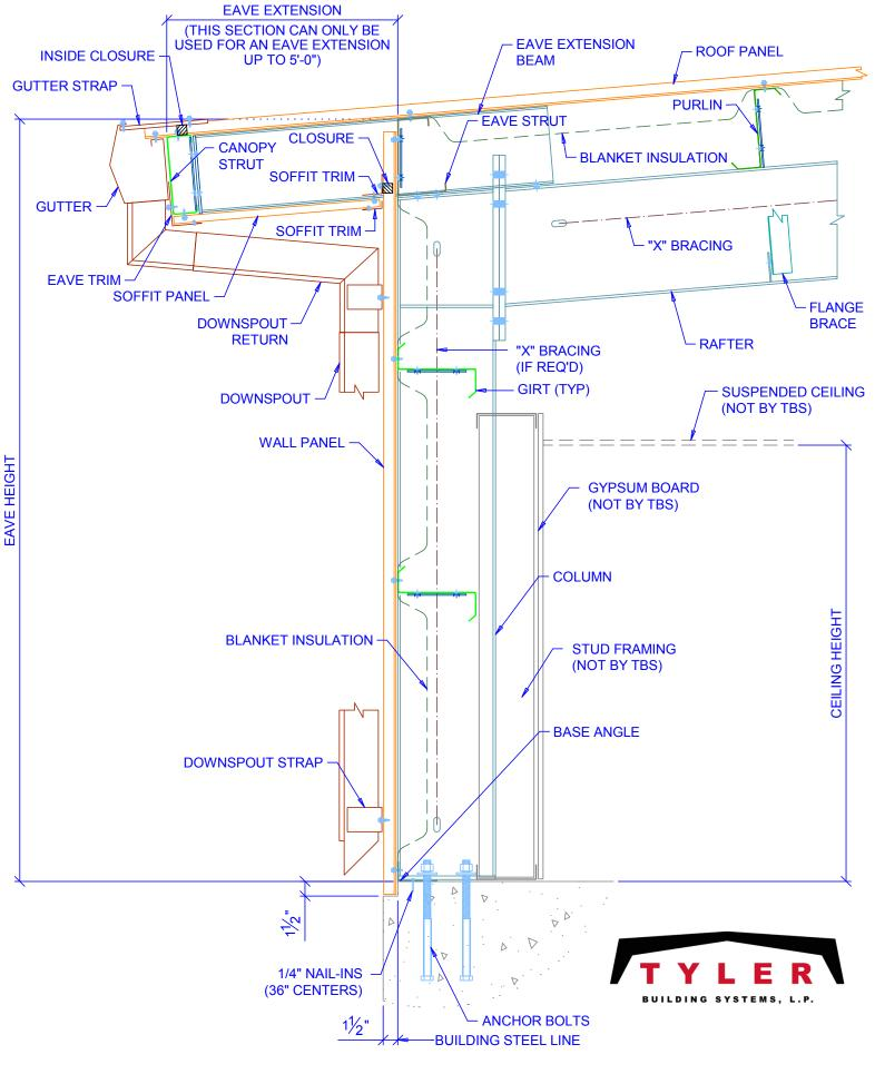
STANDARD SIDEWALL SECTION WITH STUD WALLS
