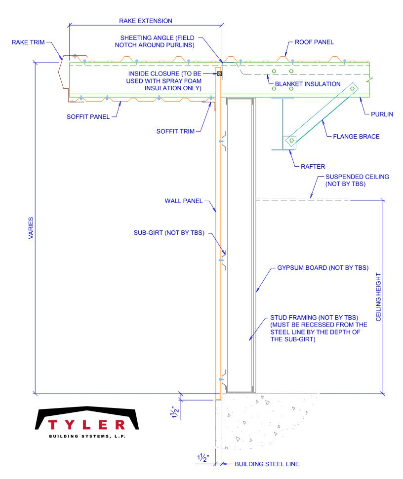
RIGID FRAME ENDWALL SECTION OPEN FOR WALL MATERIAL BY OTHERS
