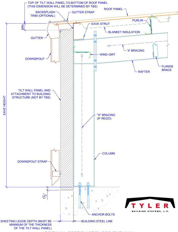
SIDEWALL SECTION OPEN FOR TILT WALL
